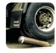
An attempt at a collision with a Standard model. The lorry wheels began spinning before it was able to run over the bollard completely.
